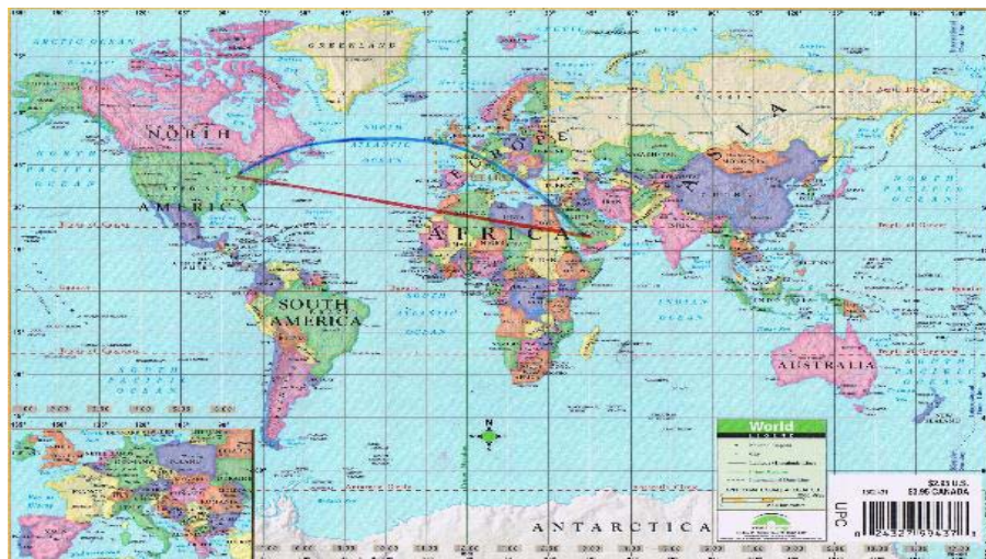
Figure 2. Great Circle line (blue: N-E direction) v.s. Rhumb line (red: S-E direction)
